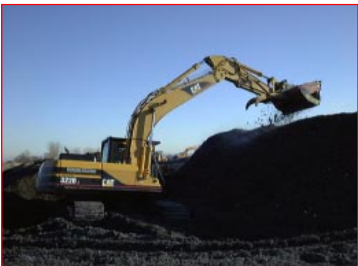
A Cat 322B excavator with an ALLU SM3-17. Screening drums can be changed quickly and easily.
