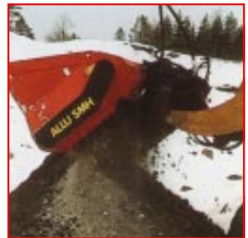
Crush lightweight concrete
