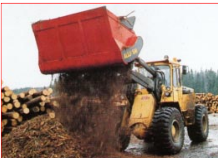
ALLU SM 3-23. The detachable adapter plate makes it quick to mount the SM units on to machines with different fastening mechanisms.
