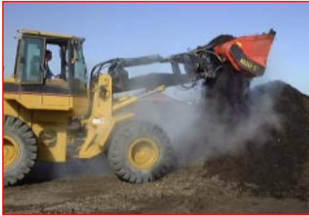
An ALLU SM3-23 (attached to a Cat IT38) busy processing compost material.
